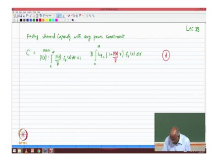
The fading channel capacity, fading channel capacity C s I t scenario with average power constraint, with average power constraint is the following problem statement; the capacity where you are allowed to choose the power allocation such that the capacity is maximized.
