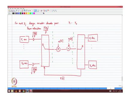
What we are going to do is since there are a finite number of gammas. So, basically for each gamma, for each gamma j design an encoder decoder pair, design the encoder decoder pair. And you also have the option of adjusting the power location. So, basically the power allocation for gamma j power allocation will be P of gamma j divided by P bar that will be the power allocation.
