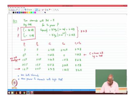
A simple example, but very illustrative in terms of the concepts that it communicates for us. There are 2 channels, 2 channels with bandwidth B width, bandwidth equal to B both channels are the same. The average SNR is the same for both, for T x power p. So that means, if I transmit with a power P on both of the channels the average SNR is going to be the same.
