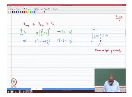
So, we will say that it is greater than or equal to gamma EGC, in general is strictly greater than no harm in saying that it is or always as good or better than selection combining. This obtains the sum of SNRs K equal to 1 through M gamma K this one achieves 1 over M summation K equal to 1 through M square root of gamma K raise whole square. And the last one is maximum of gamma 1 through gamma M.
