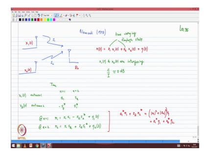
Now, I want you to think about a transmit diversity scheme which was which a very powerful scheme. So, transmitter 1 transmitter 2 this is receiver channel Z 1 Z 2.
