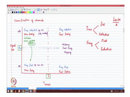
Using this the 2 parameters the coherence time and coherence bandwidth we did a four quadrant classification of channels we try to define when is it channel considered wide band when is it considered narrow band. Again a lot of it depends on the coherence bandwidth and the coherence bandwidth in turn depends on the depressiveness of the channel.
