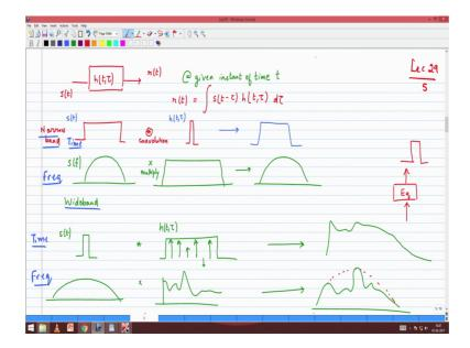
So, the multiplicative fading you have to do convolution in frequency whereas, the depressiveness of the channel results in a convolution operation in the time domain which means that it is a multiplication and the frequency domain. So, if it is a narrow band signal the depressiveness of the channel is much less than the duration of a symbol slight distortion of the of the transmitted symbol and therefore, the spectrum more or less is transmitted without much change.
