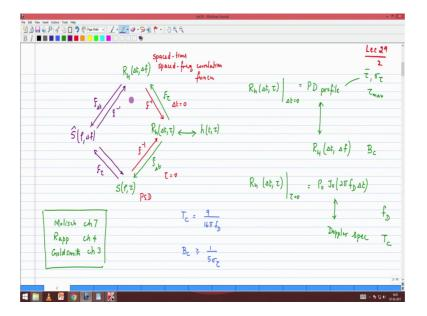
So, starting with the time varying impulse response you compute the autocorrelation function and then its 2 transforms and then the interpretations that that come from there. These are the reference points I would like you to look at and make sure that you are comfortable with that.
