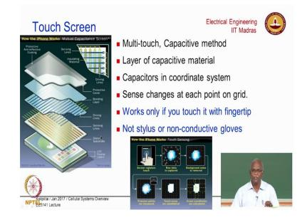
And it is like wait a minute do you know what is behind that touch screen phone it is not just oh it is working. So, here is your display, on top of that there are two layers which actually form a matrix of connections and then after that there are several layers of bonding and then finally, a protective layer. So, now, when you touch the point what it generates using this grid is it is region of locations where the contact gets made.
