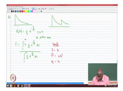
So, one of the common power delay profiles that we will encounter in wireless channels is the exponential power delay profile. So, which means that initially the signal strength is strong and then as time goes on these the delay the components delay die out, this a very common one.
