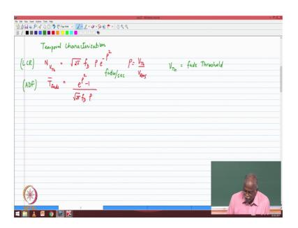
This is the level crossing rate LCR denoted by N v or n V T h basically a threshold where you declared that be the fade threshold. So, V T h is your threshold for fade if the envelop goes below that then you declare the signal to be in a fade. So, that is the and this was the what we derived in the last class was the number of basically the way of counting the fades and the average duration of a fade. So, what would be the units of N
