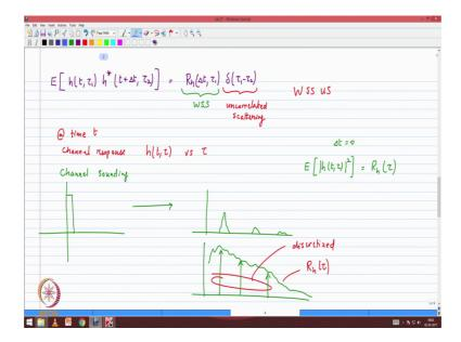
So, the argument that was made was that the interacting objects which create the multi path component at tau 1 are different from that which creates a tau 2. So, therefore, that the there is no correlation between them. So, therefore, the expression for the autocorrelation where I have t comma tau 1 h star, h of t plus delta t comma tau 2 basically boils down to the autocorrelation that we have when we had only a single tap delta times tau 1 minus tau 2.
