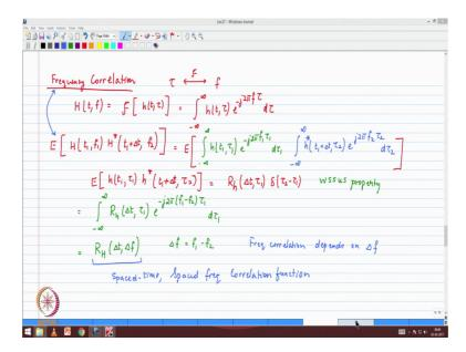
And that we will do using frequency correlation frequency correlation and the name will become clearer once we do the calculation. The first step that we are going to do is in the basically now keep in mind that we are trying to characterize the tau dimension. So, I am going to do a Fourier transform so that there is going to be a change of variables basically I do the Fourier transform for the tau dimension not the delta t, delta t is already completed.
