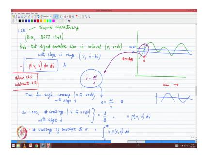
So, the LCR is the first thing that we will address- level crossing rate. The original formulation of this by the way this is another aspect of the temporal characterization, just write that down. This is also part of the temporal characterization; this also has to deal with the variation with respect to the function t of variable t and not tau this is variable t.
