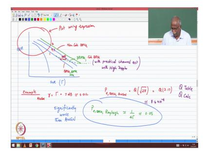
So, here is my bit error rate as a function of SNR, notice that I can now write it in terms of the SNR as gamma or E b by N naught average value AWGN graph is going to be steep this is BPSK; this is differential BPSK. So, this one is BPSK the shift of 3 d B and this is going to be differential BPSK and why is d BPSK worse than BPSK because of the.
