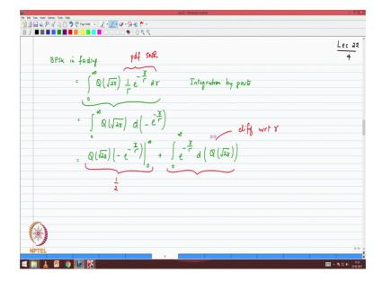
Now, we moved over from there to BPSK and we wrote down the expression for the bit error rate in fading which involved the Q function and the distribution of SNR again we will use the SNR distribution. So, that is the p d f of the SNR we did the first step of integration by parts and I hope you had a chance to complete the step that we had where we left of and we showed that the integration by parts actually results in a derivative of an integral.
