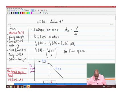
So the summary that came from lecture 6 break point model states I will take free space propagation up to the break point; that means, from the source antenna radiation point up to break point, and then go at a slop that is greater than two because of a higher path loos. So, basically this is receive signal power as a function log d logarithmic that that is when you get the straight lines. So, this is the break point model and we looked at some calculations using the break point model.
