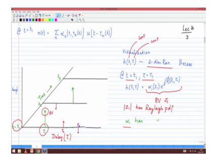
One of the very useful ways of equalization of a multipath channel is to think of it in terms of two dimensions; one dimension being the delay dimension, the other one being the time dimension. So, at any given point, if you take a snapshot, you get a certain multipath profile basically number of multipath components at the delays, the gains are occurring. We have shown a few examples. Now, basically this is a visualization of what is in reality a continuous function.
