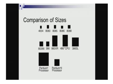
And when you see the comparison of sizes of the die please note that the die size has not grown very big, but the number of transistors that we put inside a die that this transistors per unit area has significantly increased and that is the integrated circuit revolution.
