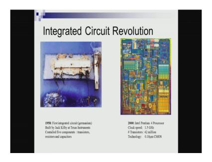
The first thing that we are we should note is the major integrated circuit revolution which came in 1958 from Jack Kilby of Texas instruments where he showed that on a same substrate more than one component can coexist. So, he made one substrate where it had 5 components there a couple of transistors resistors and capacitors all of them existed on the same substrate what you see on your left hand side in your screen.
