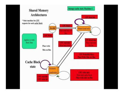
And now this is one state machine the largest state machine, this is the state machine for CPU request there is the snoopy cache state machine 1. This is something because of my processor, this is what happens to your state of a particular cache line based on it is own processor trying to read or write from the memory.
