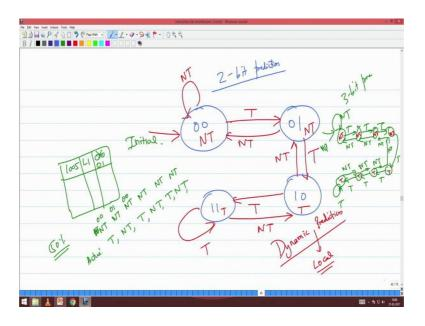
So, we will continue our discussion on branch prediction. So, last class we saw at two bit branch predictor the way it works and I also extended it into three bit and n bit. And we also stopped with one statement which was empirically proved statement saying that a two bit predictor works as good as a n bit predictor.
