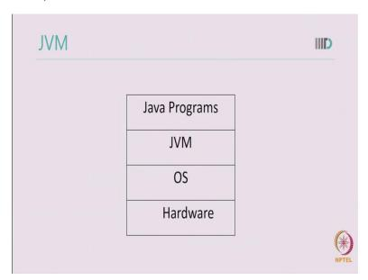
This is a simple structure showing how the java program lives on a given machine. You may have a hardware on top of the hardware you may have different OS. For example Linux, windows or mac operating system. You have a different JVM for different Operating systems. And then you have a java programs. As a developer you write a java program and then JVM hides all the complexity of the underline operating system to hardware from you.
