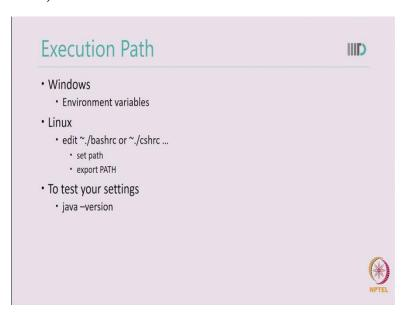
After you have downloaded java on your platform you will have to Set the path correctly so that your system can recognize java program in windows operating (sys) in windows operating system you do it using environment variable in Linux you do it by bashrc or cshrc files or other shell files that you may be using. You can test your setting by running java – version command.
