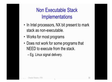
In Intel machines, an NX bit is present in the page tables to mark the stack as nonexecutable. While this work for most of the programs that is in most programs it is a added benefit, but the problem is some programs even though they need not be malicious require to execute from the stack. These programs need to execute from the stack in order to function properly. Therefore, setting the NX bit is not always very beneficial for all programs.
