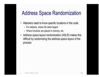
Another way to prevent this particular attack something known as the address space randomization or ASLR, in this particular counter measure technique it uses the fact that the attackers need to know specific locations in the code. In the return to lib c attack for instance, the attacker needed to know where the function F 1 or in our example where the function system was located in the program space. N
