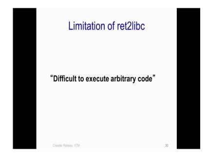
Now, the limitation of the return to lib c is that it is extremely difficult to execute some arbitrary code. So, we have seen one example of how the attacker could execute a shell, but the amount that an attacker could do with the return to libc type of attack is very limited. And therefore, the attacks over the period of time have evolved to something stronger.
