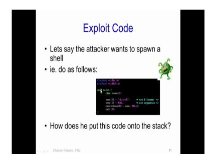
So, now we will see how a one particular attack code is created, and how an attacker can force an application or an operating system to execute that exploit code. Let us take a very simple example of the exploit code, which is shown over here. Essentially this exploit code which we call as shell code does nothing but only executes a particular shell, the shell is specified by slash bin slash sh.
