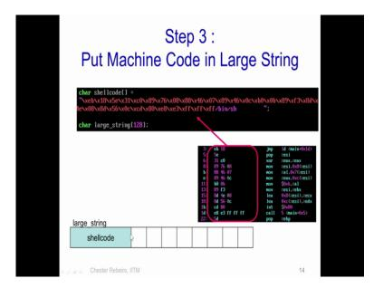
So, what the attacker would then do is create something known as the shell code array which essentially is the code that he wants to execute. So, he creates the shell code array comprising of all the assembly up codes or machine codes which it wants to execute and he places this code or the shell code in the first part of the large string. So, if you look at this the large string array, which is a very large string of 128 bytes in this case, gets the shell code in the first part.
