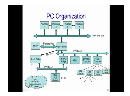
So, this particular slide here shows how a typical PC is organized. So, we may have multiple processors present in the system. So, this could be 1 processor, 2 processor, 3 or 4 and so on. So, it could also be possible that each of this processor have multiple cores inside them; and each core has 2 or 4 threads. Now all these processors are connected to each other through what is known as the front side bus. So, there is always a sharing
