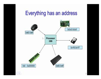
Essentially, each device in the system would have a unique address. And it is ensured that no two devices in the system would have the same address. For instance, we would have the hard disk which is present from the address range 0x1f0 to 0x1f7. So, what this means is that when the processor sends out an address on its address bus, the hard disk would identify that the address is within this particular range and therefore, it will respond.
