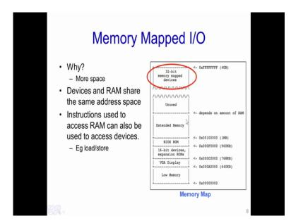
In order to extend this, what was used was known as the memory mapped IO. In this particular memory mapped IO, hardware devices would then connect or would be then mapped into regions in the memory addressing itself. As we have seen before, the RAM or the random access memory of the system would be addressed from the location 0 and extend upwards until the end of the RAM.
