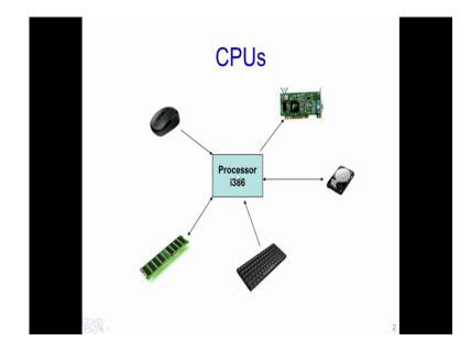
So ,we know that the heart of any system is the CPU; and the CPU is interfaced to several devices such as the VGA card, a hard disk, a keyboard, RAM, mouse and so on. Now, in order that all these devices work with single processors - what is required, is addresses.
