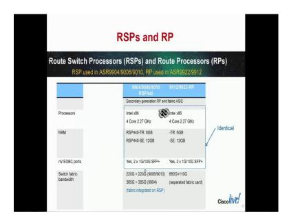
Now, usually this is Route Switch Processor, you can have a general purpose processor. Usually, x86 4 core 2.27 is actually used in 9000 process, which is actually normal that you find in your server boots but one of the things you should see is the switch fabric bandwidth, that is runs into 220 gig and so on. So, this is all data from field data not theoretical data.
