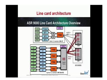
Here is ASR 9000 router; here is an example of how they are all interconnected. If you look at this case for example, this is a normal CPU. So, here it has 92 gig interface, where as with the linecard and other phase it is got 440 gig interface.
