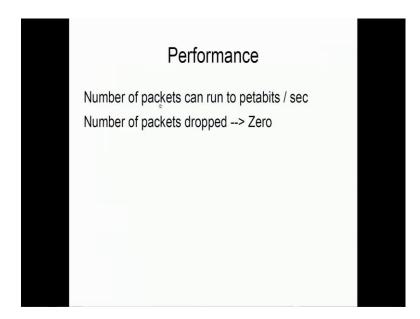
Number of packets that router can get, can go into petabits per second and then number of dropped packets should be more or less zero because in any drop packets it has to be retransmitted by top level protocols and things like that. There are lot of complications in protocols.
