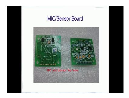
Our MIC and sensor board, this was a digital MIC that we actually use for our codec. For the calls that we are making we actually had a digital MIC instead of an analog MIC. This is the sensor board that was actually connected on to our carrier board so this had all the sensors, the proximity, the accelerometer, the gyrometer, the front and the rare cameras that we are actually used from omniview. So, these components are actually again integrated into the board.
