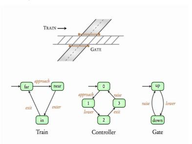
We had seen this Train Gate example in a previous unit let me recall so this is a railway crossing and there is a Gate which is controlled by a software we need to make sure that the Gate is down whenever the Train is in, let us see a model of this system. So let us start with the Train, so the Train is initially far that's denoted by this far state when its approaching close to the crossing it senses a signal approach and comes to the state near this means that it is near the crossing.
