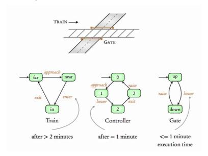
Let us see how to do it firstly, based on the speed of the Train and other physical properties we can make certain assumptions about the time taken for the Train between approach and the enter signal okay, assume that once the Train sense the approach signal to the Gate it takes
