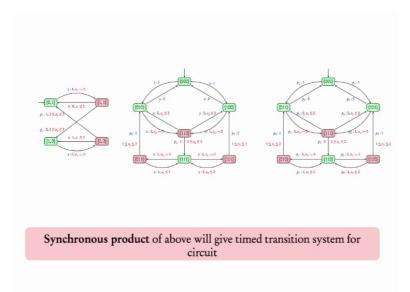
Now the synchronous product of these three Timed transition systems whether give us the time transition system for the entire circuit and the synchronization is happening through this actions for example this one says that x is becoming 1 and here there will be synchronizations on if x becomes 1 what to do on so on.
