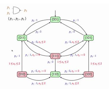
Now you can also do the same thing for this Gate for this Gate you have two inputs and one output so a state is given by value of x, y and p 2 so there are eight states however one of the states was not reachable so we have not written that so see 000 matches the truth table so this is stable however 110 does not match the truth table which is unstable. You can go through the transitions and see that they match the inertial delay of 1, 3 for this Gate.
