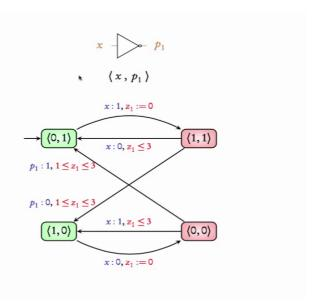
So let us start with the NOT Gate it has a timing delay 1, 3 now how do we give the state of this NOT Gate the state is given by the value of the input the current value of the input and the current value of the output so x, p 1 and there are four possibilities the red ones are the unstable states, the green ones are the stable states.
