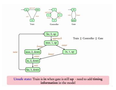
The joint behaviour is given by this handshake operator which is some synchronous product so from far, 0, up when there is an approach far goes to near and 0 goes to 1 okay, that's the state change so based on this idea this is the transition system of the joint behaviour, if you see there is a way in which the Train can be in, but still the Gate is up, this is not a safe state.
