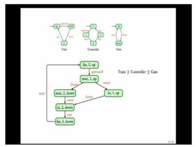
This is the transition system representing joint behavior of the train controller and gate. Approach, exit, lower, raise are handshake actions. Approach a shared between train and controller, raise a shared between controller and gate and so on. Initially the joint state is given by far 0 up approach is possible from the train and controller. So on an approach both the train and the controller change state.
