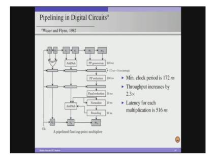
So, we know that the multiplication part. The multiplication of these mantissa components consists of three portions; one is the partial product generation, partial product reduction and final reduction. And each is taking 125ns, 150ns and 55ns respectively. And the next one is normalization which is going to take 20ns and rounding is going to take 50ns. Now, given
