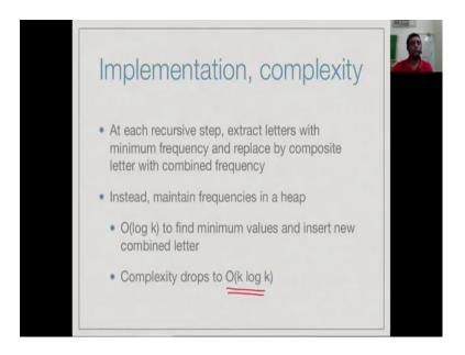
So, if I maintain the frequencies is not at as a heap, then the order log k time, I can find the minimum values and then I can insert back the new composite letter also into heap in to log k time. So, each iteration takes some log k, and so I am improving from k square to k log k.
