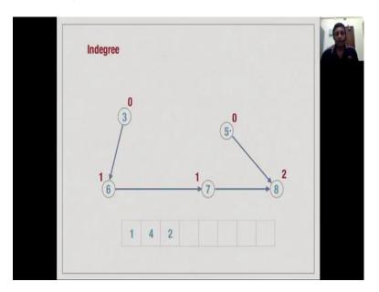
So, when you do pass 2 then the in degree of 3 reduces and the in degree of 8 again reduces. So, notice that 8 still has to pending in requirements only 5 and 7, so it cannot be done yet, but 3 and 5 are the available.
