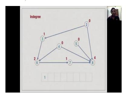
So, what happens on eliminate 1 is that we enumerated and we reduce the in degrees of 3, 4 and 5 from 2, 1 1 to 1 0 0.
