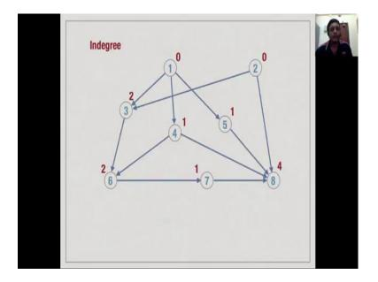
So, let us apply the strategy to this DAG, so we first begin by labelling every vertex by it is in degree. So, will read we have indicated the in degree of the every vertex. So, for instance 1 and 2 have no incoming edges. So, they have in degree 0, vertex 3 as 2 edges coming as in degree 2, vertex 8 has 4 edges coming inside and in degree as 4 and so on, now we have to pick up a vertex of in degree 0 enumerated and eliminated.
