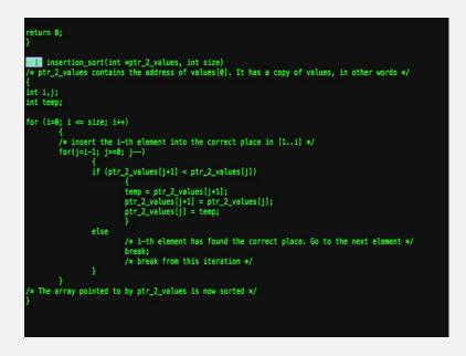
So, the function is called insertion sort and it does not return any value that is why you see the void here. Now, observe that the data type of the first argument is a pointer to integer and you will already recognize that the variable pointer to values contains the address of values of 0. Whenever this function called is made, when control enters this function ptr underscore 2 underscore values contains the address of values of 0.
