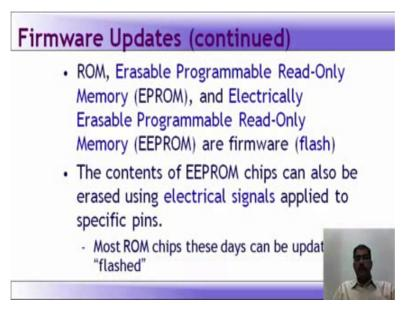
ROM, erasable programmable read only memory EPROM and electrically erasable programmable read only memory EEPROM are firmware or flash devices or flash. The contents of EPROM chips can also be erased using electrical signals applied to specific pins. Most ROM chips these days can be updated or you would have hear the terminology flashed. In say some fifteen years back, the desktops that were purchased do
