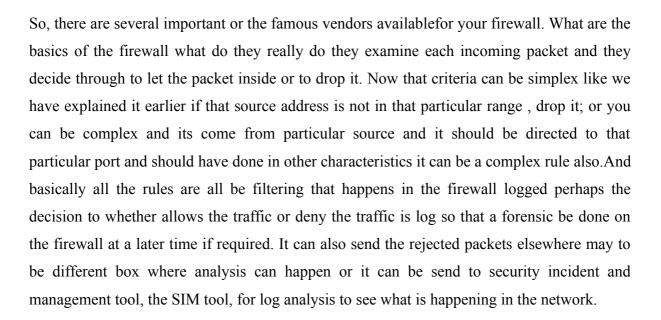
So, basically this are the functions for the basic properties of firewall it also complex than that, but what we need to understand is it examines each packet then it decides that to allow the packet in or to drop the packet or it could send the packet somewhere else, it logs all the traffic coming in if you configure it this criteria appropriate can be simple process or a complex process.
