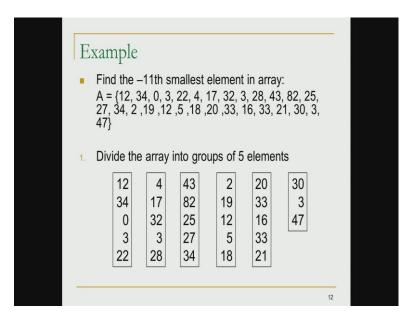
Let us run through an example of this algorithm. In the given array of 28 elements, we want to find the eleventh ranked element. In the first step we divide the array into 5 groups of 5 elements each which may counts for 25 elements, and 1 group the last group of 3 elements.
