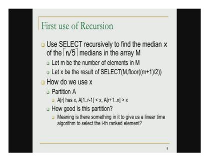
Now, we here is the first use of recursion. We look at the array m and ask for the median of the n by 5 elements in the array M. So, the recursive call is described here, if there are m elements in the array, then the recursive call is select on the array m, the median element which we know is floor of m plus 1 by 2, let the returned value be x. Now what we do is the partition the array A into 2 parts around the element x. We will see how to
