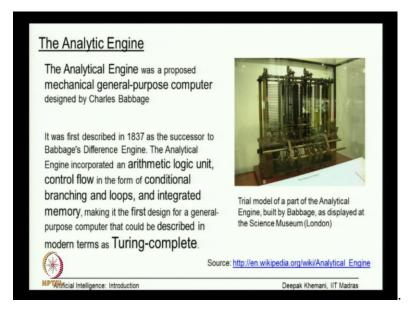
And he created what is known as the analytic engine. It was a proposed, he did not actually build it, mechanical general purpose computer designed by Charles Babbage, first describe in 1837. It had an arithmetical logic unit control flow, all modern terms in computer science in the form of conditional and branching loops and integrated memory. And, it was the first machine which in the modern sense could be said to be Turing-complete which means it is equivalent to a Turing machine.
