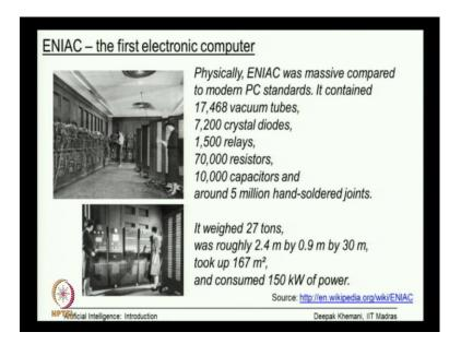
And finally, in this study of mechanical history we look at this first electronic machine which was built called ENIAC. You must be familiar with it. And, you can just see the size of ENIAC - 17,000 vacuum tubes, 7, 200 crystal diodes, and so on and so forth. 27 tons, it occupied a full room essentially. It was not even as powerful as a small computer that you have on a smart phone nowadays. But, that was the first electronic machine essentially.
