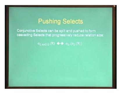
The second form of rewriting rules is also related to pushing selects and which is called the cascading select or conjunctive selects. That is a select which has a conjunction can be split and cascaded into several different select operations and which can progressively start reducing the search space as we go along. This slide shows a small example which illustrates this point.
