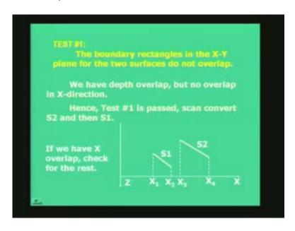
So test one is passed in this case and you scan convert S2 and then S1. If you have an X overlap check for the second test or the rest of the test. So go to test number two, what does test number two say? Surface S is completely behind the overlapping surface relative to the viewing position. That is what you do in test number two. But let us look at this figure and understand why we have come to test number two at all.
