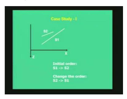
I hope you have understood why test number two fails because for the test number two to succeed S1should have been completely behind surface S2 which is not possible in this case so test number two also fails.
