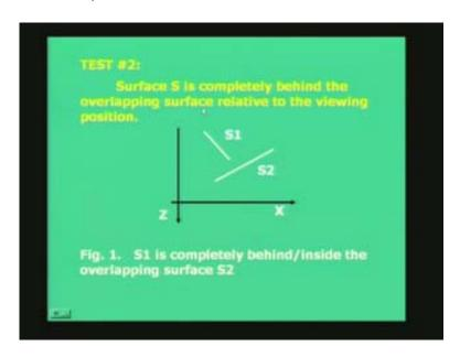
Let us look into the scenario where test number two will fail. To do that we look into this figure here. Why does test number two fails and that is why we have to go to test number three. S1 is not completely behind S2 as you can see here now. You check this figure and you will see that
