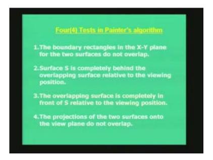
The test two says that the surface S which is under test is completely behind the overlapping surface relating to the viewing direction. We will see the surface S which has to be rendered first whether it is completely behind the overlapping surface. We will see what this behind test is all about and how it is done. If this test also fails we move on test number three where we will say that the overlapping surface is completely in front of S relative to the viewing position.
