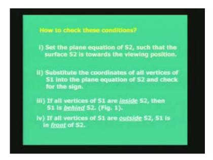
And if all vertices of S1 are outside S2 S1 is in front of S2 this is with respect to figure two. So if all vertices of S1 are outside S2 then this is the simple way of substituting vertex into the other equation and that is what you do to check this condition. Now, going forward and looking into test number four. We enter this test only when test number zero one two and three all of them fail.
