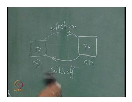
Now, apart from this let us consider a simple 1 suppose you are having a Tv and when you switch switch on the switch on switch switch on the Tv is initially off, then when you switch on it goes to the on stage; when you switch off it goes to the off stage is a small instance of a day to day life which you can a represent it by means of a state diagram like this.
