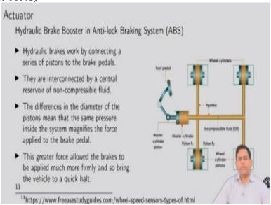
So, continue from there. So, here is just a simple example of an actuator. So, it is basically the hydraulic brake booster which is very much standard in antilock braking systems in automotive. Now all of us are quite aware of the physics principles how I mean in a hydraulic system you have liquids which can amplify the pressure right. So, this breaking principle of the actuator is primarily based on that.
