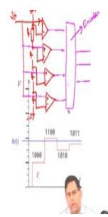
So let us take an example here. So here we have an example of ADC algorithm which of course will be implemented in hardware. And let us understand that how I can convert this analog signal to a corresponding sequence of bits which will be transmitted to a digital computer. So, the idea here is of one of successive approximation so what happens is suppose we are trying to reach we are trying to approximately represent this analog value, okay.
