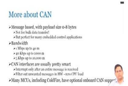
Now of course, the bandwidth has a limitation on the cable length. We can understand that from simple physics here. So, if you are trying to afford 1 Mbps speed, your cable end to end length should be inside 40 meter. Similarly, for something some limit for 40 kbps or slower speed higher range much, I mean, something like 5 kbps much slower speed you can have a much bigger cable.
