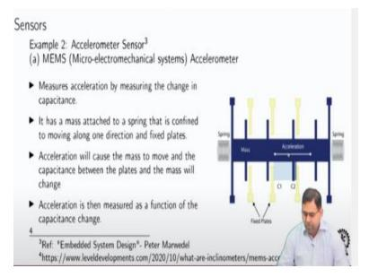
So, we will start with the accelerometer sensor. We are taking an example of a MEMS accelerometer here. MEMS full form is Micro-electromechanical system accelerometer. So, let us see. So, like we said that the accelerometer, what it does is? It measures the velocity or in other way the linear acceleration in the different directions, right. So, this kind of Micro-electromechanical accelerator, what it does is? It will be measuring the acceleration using change in capacitance.
