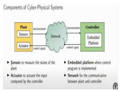
So here we have a simple high-level model of a CPS and which is trying to tell you that what are, the rules that sensors and actuators play. So as you can see that there are sensors which are gathering measurements and they are sending those measurements over the network. There is a control software which is running on an embedded platform and that is using these sensed values to create a control action.
