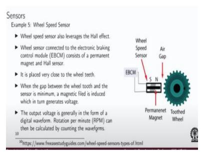
So, this principle is very commonly used in the wheel speed sensor of vehicles. So, what they do is, they will attach a wheel like this. So, they will attach a wheel like this in the wheel well and then they will have this kind of permanent magnet. And there will be air gap and this is the wheel that is there with teeth, right. So, when this wheel is rotating at some speed, in a proportionally a number of teeth crossing this magnet will keep on changing, right.
