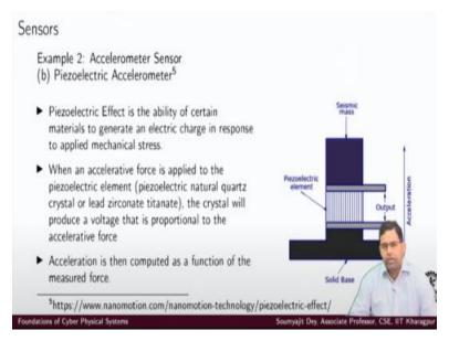
Similarly, we can have accelerometers based on piezoelectric. So, piezoelectric as we know they have the ability to generate an electric charge in response to some mechanical stress that is applied, right. So, if you put pressure on a piezoelectric crystal, it will generate an electric charge, right. So, let us say you have a seismic mass here, right and you have this piezoelectric element. Now you give some acceleration here if and this is a solid base.
