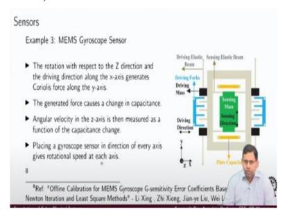
You can also have MEMS gyroscope sensors right. So, what they do is again, they have a principle of changing capacitance. With respect to this change in capacitance you can actually measure this velocity in the in the different directions. So, when this gyroscope is rotating with respect to the Z direction and there is a, and the driving direction along the X axis it will generate a Coriolis force along the Y axis.
