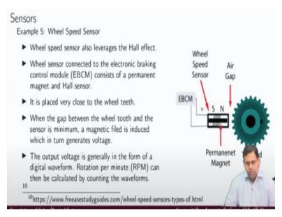
Now something about sensors, so we spoke about several different kinds of sensors that are used we talked about IMU sensor in general, which actually contains the linear acceleration sensors, the orientation sensors, the gravity sensor. And then we talked about some accelerometer system using capacitances which can be used for sensing the acceleration. Then we also talked about accelerometers which can be built using piezoelectric crystals.
