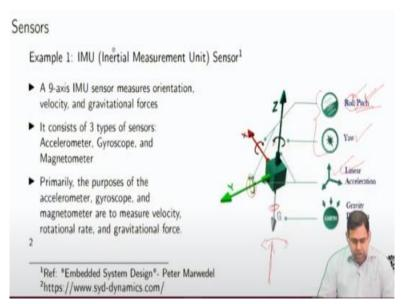
So, we will just have some introduction on different sensors. So, we will just list a set of popular sensors that are typically used. For example, we will talk about IMU sensors Inertial Measurement Unit full form. That is the Inertial Measurement Unit the acronym is IMU. You must have heard of this. This IMU sensors because they are nowadays kind of ubiquitous around us right. They are part of so many different kinds of devices around us.
