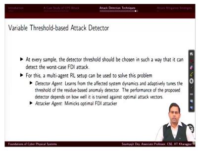
And what we can do is at every sample the threshold detector would choose in such a way that it can detect the worst-case FDI attack. That means ah we are looking at estimating what is the worst-case attack. At every cycle dynamically I am trying to see what can be the attack that can happen? And then into truth word that I will like to choose suitable values, suitable parameters for the detector.
