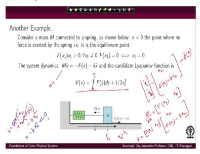
Now, let us take another example ah from the same material we have been covering here. So, we have a spring mass system, ah of mass M. right. It is connected to the spring ah and x equal to 0 is the point when no force is exerted by the spring ah since by this spring. Right. So that is
