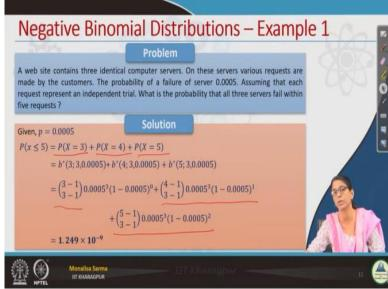
So we will see an example a website contains 3 identical computer servers on this servers various requests are made by the customer the probability of a failure of server is 0.0005. The probability of there is a probability failure assuming that each request represents an independent trial here also trials are independent like what we have seen in binomial distribution, what is the probability that all 3 servers fails within 5 requests?
