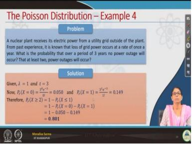
So, 1 more example here we have a nuclear plant receives this electric power from a utility grid outside of the plant. From past experience, it is known that loss of grid powers occurs at a rate of once a year. A nuclear plant receives its electric power from a utility grid outside of the plant, from past experience, it is known that loss of grid occurs at a rate of once a year. So that is  $\lambda$  average is once a year  $\lambda$  is 1 per year.
