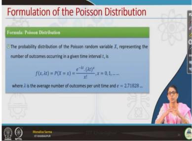
Now, what is the function of Poisson distribution and Poisson distribution we have a parameter that is we call it lambda where lambda is the average number of outcomes per unit time, average number of cars passing through that highway in 1 hour. average number of cars passing the toll station in 1 hour or in 24 hours, whatever it is, so that is the parameter this is lambda.
