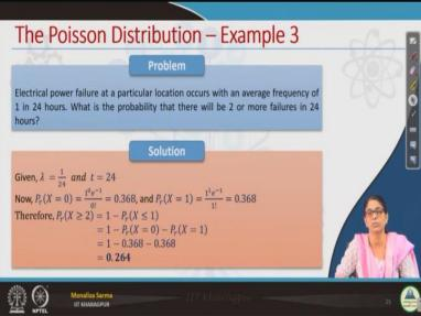
So, now, 1 small example, electrical power failure at a particular location occurs with an average frequency of 1 in 24 hours, what is the probability that there will be 2 or more failures in 24 hours? What it is given every frequency is 1 in 24 hours that means  $\lambda$  is 1 per 24 hours. Now, what we need to find out what is the probability that there will be 2 or more failure in 24 hours? My t is 24 hours and I have found in  $\lambda$  also 1 in 24 hours.
