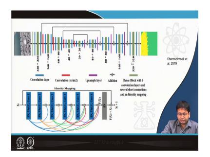
So, the task here is to separate like. So, this is again as you can see this is again has a U-Net kind of structure with multiple skip connections like this and so, like they one important aspect or one important addition they have made on top of it is something known as identity mapping.
