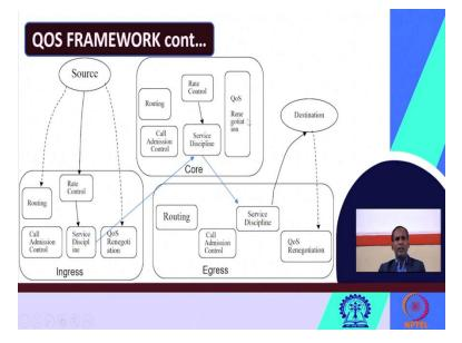
Now, let us quickly look what the QoS framework, there are several components which work to provide QoS support to a connection request. So, these components can be treated as the elements of QoS framework. You can see the QoS framework can look like this. So, this is the source and this is the destination you see the major components are what call admission control, rate control, service discipline, QoS renegotiation.
