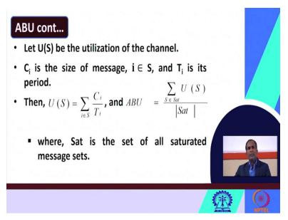
So, let us see an mathematical expression for a view let us assume that the U(S) be the utilization of the channel. Let U(S) represents the utilization of the channel, Ci represents the size of the message where i  $\epsilon$ S and the Ti is its period. Then utilization of the channel U(S) can be defined as  $\sum_{i \epsilon S}$ Ci / Ti. So, what is Ci / Ti we have already known this in the utilization Ci the size of the message where Ti is its period.
