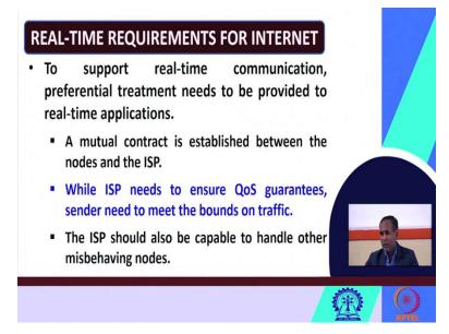
So, the real time requirements for internet let us see what are the basic real time requirements. To support real time communication preferential treatment needs to be provided to the real time application. So, the preferential treatment needs to be provided to the real time applications a mutual contract established between the nodes and the ISP. So, to support real time communication a mutual contract has to be established between the different nodes and the ISP the internet service provider.
