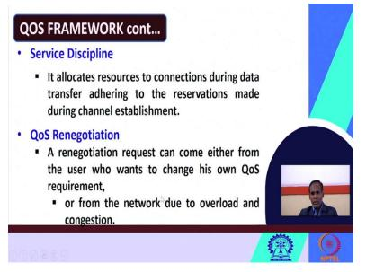
Then the next one is service discipline? What does this component do? This component allocates resources to the connections during data transfer adhering to the reservations made during channel establishment. So, as its name suggests service discipline, it allocates what? It allocates the resources, to whom? To the connections, when? During the data transfer adhering to the reservations which are made during the channel establishment.
