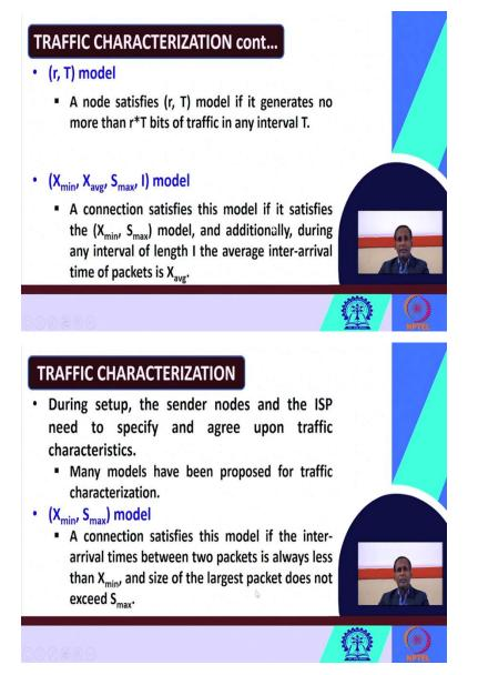
Then you will see the next model called as r T model, a node satisfies this model r T model if this generates no more than r into T number of bits of traffic in any interval t. So, any node will say that it satisfies r T model if it does not generate more than r into T number of bits of traffic during or any interval T. Next model is the X min, X average, S max and I model. A network connection satisfies this model if it is satisfying the following.
