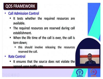
First, we will see call admission control. What does this component represent should this component call admission control it tests whether the required resources are available or not. So, this component call admission control. It tests whether the required resources are available or not, the required resources are reserved during call establishment. All the required resources they are reserved during on the call establishment.
