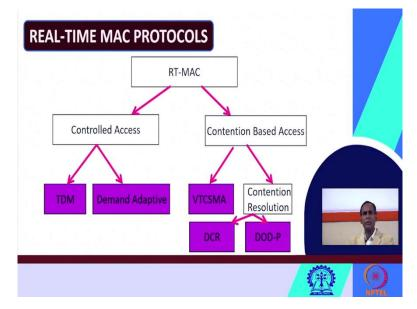
I have already told you real time MAC protocols can be divided into two categories; one is contention-based access; another is contention free access or controlled access. Under controlled access you can see the examples are TDM or round robin another is demand adaptive. And in contention-based access you can see that what categories are VTCSMA which is a variation of CSMA and another contention resolution.
