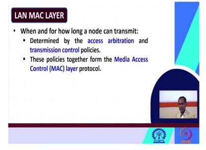
So, we will see that LAN MAC layer, so, when and for how long a node can transmit so in a LAN for what period of time a node can transmit and when it can start transmission how to decide. So, this thing is decided is determined by two important policies, two important processes; one is access arbitration policy another is transmission control policy. When a node can transmit and for how long duration a node can n transmit this can be determined by the access arbitration by two policies.
