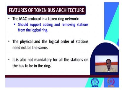
So, some of the features of token bus architecture you can see. So, in case of token architecture, the MAC protocol in the token ring network it should support adding and removing station from the logical ring. So, I have already told you in token bus architecture the stations maybe arranged in the form of a logical ring. The MAC protocol in case of a token in network it should support adding and removing stations.
