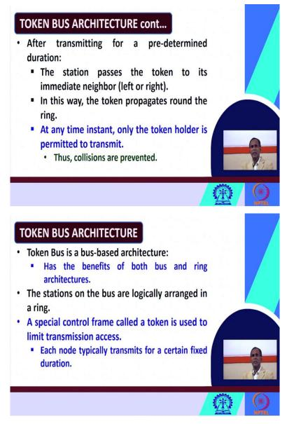
So, after transmission for a predetermined duration the station passes the token to the immediate neighbour. So, when I have already told you here each node uses a certain fixed duration. So, now after transmitting for that pre-determine duration for that specific duration then this station what does it do? Then this station passes the token to whom? To its immediate neighbour that immediate neighbour may be on the left-hand side or on the right-hand side.
