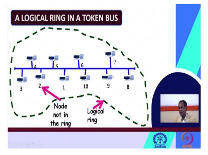
See here I have a just shown a token bus architecture you can see a logical ring is formed, you can just a little bit of what, the my diagram is not correct like this 7 is here it is present in the ring. Similarly, can see actually this ring is not, this logical ring is a little bit mistake I have while I have drawn, so like 3 it can be there, but you see 2 it is not there in the ring.
