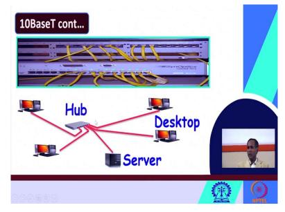
This is a sample figure of this 10BaseT you see all the nodes how they are connected to a hub. See all the servers, desktop, these are the nodes they are connected to a hub in 10BaseT ethernet.
