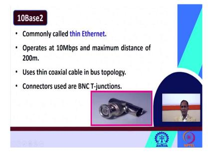
So, 10Base2 it is commonly called as thin ethernet and this 10Base2 this thin ethernet operates at 10 Mbps and its maximum distance and at maximum distance of 200 meter. Please remember this is very important. 10Base2 is known as thin ethernet. It operates at 10 Mbps speed and at maximum distance of 200 meters only. What does it use? It uses thin coaxial cable this 10Base2 it uses thin coaxial cable in bus topology.
