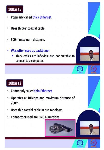
Similarly, you can understand yourself about 10Base5. So, 10Base5 it is popularly known as thick ethernet. 10Base2 is known as thin ethernet, 10Base5 is known as thick ethernet and it uses a thicker coaxial cable. So, 10Base2 uses thinner coaxial cable. But is uses a thinner coaxial cable, but it uses a, what? Thinner coaxial cable. But 10Base5 uses a thicker coaxial cable and the maximum distance is 500 meter here.
