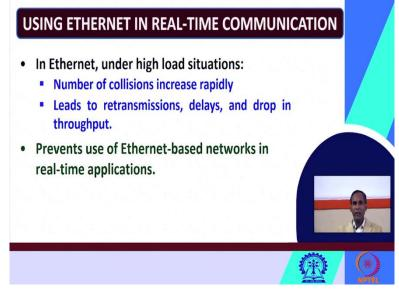
So, the now on the using ethernet in real time communication what is the drawback? How far it is suitable to be used in real time communication? In ethernet under high load situations the number of collisions they increase very rapidly. This will lead to retransmission and the delays and drop in throughput, I am repeating again what is the problem if you will use ethernet in real time communication.
