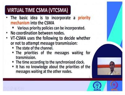
So, now let us see about the first one VTCSMA under contention-based approach. VTCSMA, it stands for what I can say V stands for virtual, T stands for time. So, this is virtual time CSMA. Here the basic idea is to incorporate a priority mechanism into the CSMA. Here the basic idea is to incorporate what? A priority mechanism. How to incorporate a priority mechanism into the CSMA?
