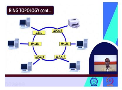
Now let us see what is the problem? What are the limitations? What are the limitations of ring architecture? First, the important problems with the ring network are as follows. First drawback, any break in the ring can bring the whole network down. You see if any node is broken, is faulty, then what will happen? The whole ring will fail. So, any break in the link can totally bring the whole network down.
