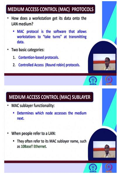
Now let us see first, a little bit more about the medium access control protocols. I have already told you so here in the functionality of MAC sublayer is that it determines which node accesses the medium next so how does a workstation gets its data onto the LAN medium? How does the workstation or a node gets its data onto the land medium? So, MAC protocol, by using the MAC protocol it can be done. So, how does a workstation gets its data onto the LAN medium?
