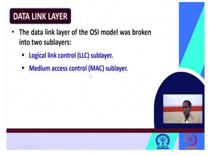
Before going to the details of the ethernet let us quickly look at this data link layer you know that OSI model it has 7 layers starting from the at bottom you can see physical layer, data link layer then like that and the topmost layer is the application layer. So, in data link layer, the data link layer of the OSI model was broken into two sub layers. So, I have already told you after this physical layer then this data link layer.
