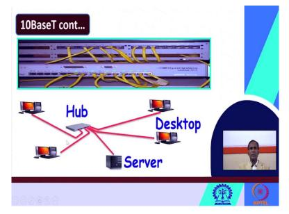
Next we will quickly go to this 10 Mbps ethernet. The difference variations I have already told you 10Base2, 10Base5, 10BaseT and similarly another is F. In 10Base5 we use thick coaxial cable, maximum distance is a 5-meter, number of nodes can be connected is 100 and advantage is it is used for backbones. In 10Base2 it uses a thin coaxial cable, maximum distance is 200 meter, number of nodes can be connected 30 and advantage is cheapest.
