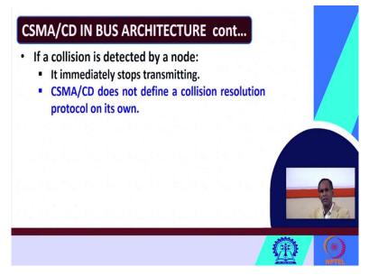
So, if we will see that if a collision is detected by a node, then what it will do? So, when in CSMA CD it detected that if a collision is detected by a node, then what happens the node immediately stops transmitting. The node it stops the transmitting process then CSMA CD does not define a collision resolution protocol on its own.
