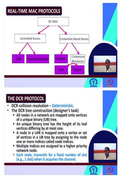
Then we will see the next category which is coming under this one contention resolution DCR and DOD-P. So, DCR stands for D stands for what deterministic, C, collision, R is resolution. So, DCR protocol it stands for deterministic collision resolution Protocol. So, basically DCR is a deterministic collision resolution protocol. Here in DCR a tree is constructed we call it as DCR tree.
