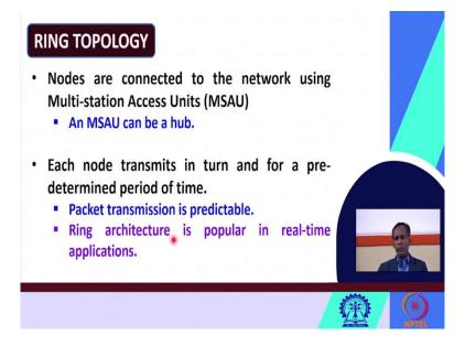
So, then quickly we will look at ring topology, here the nodes are connected to the network using multi-station access units, we call it MSAU, so what could be an MSAU? An MSAU can be any hub, so here each node transmits in turn, in ring topology what happens? Each node it transmits in turn and for a particular point for a particular duration of time.
