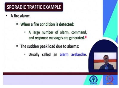
You can take the example, good example of the fire alarm system those are put in multi storied buildings. So, how does the fire alarm works? So, when a fire condition is detected, then what happens? A large number of messages are generated, for example, a large number of alarms, large number of commands and large number of response messages are generated because a fire condition a smoke is detected.
