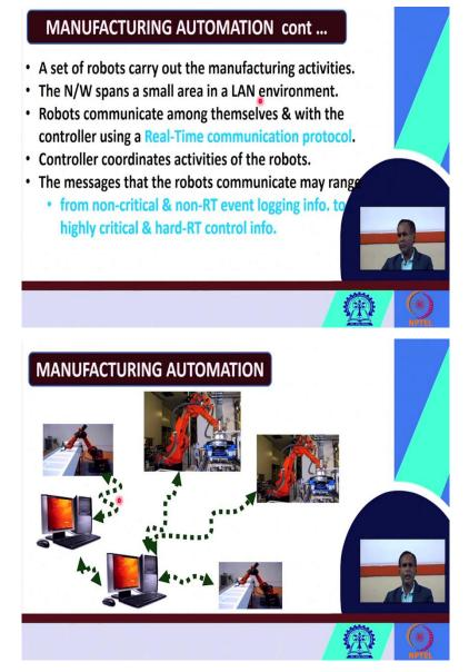
So, let us see how they in detail how these have been appearing I have already told you in manufacturing company what happens, or in manufacturing automation a set of robots they carry out the routine manufacturing activities, the network it spans a small area in a LAN environment, because it is a small company, so these robots are placed at the different locations.
