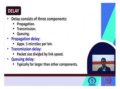
Now, let us see some of the important parameters that we have discussed in this or some maybe some important quality of service parameters in real time communication. First let us discuss about to delay. So, in real time communication the delay consists of three important components; one is propagation, next is transmission, next is queuing delay. So, propagation delay, transmission delay and the queuing delay.
