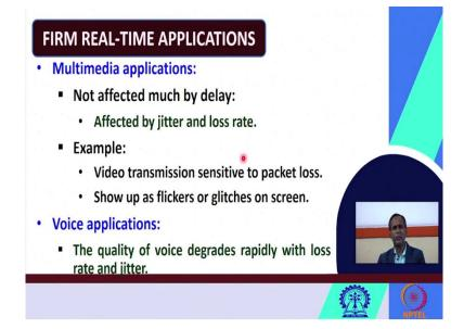
Then we have already seen the soft real time systems then we will see about something firm real time applications, how these real time communication is what addressed here. So, let us see the example or the cases of the firm real time applications where the real time communication is applied how it is applied. So, you know the best time examples of firm real time applications are what? The multimedia applications, voice applications etcetera.
