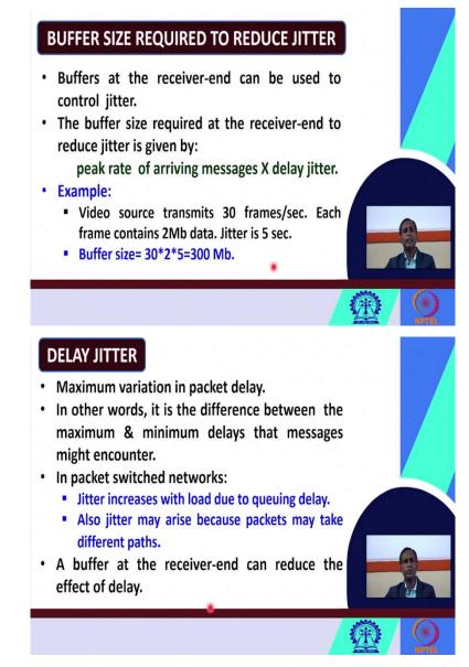
So, now let us see how we can estimate what should be buffer, size of the buffer that we want to put I have already told you, a buffer at the receiver end it can reduce the effect of delay, now then how we should know? What should this size of the buffer that will be put on the receiver end. So, that is a formula that we can calculate what should be the size of the buffer that is required to reduce the jitter.
