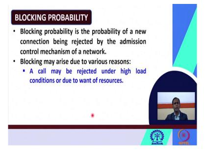
We will see one more case parameter that is blocking probability. Now, let us see how blocking probability is defined. Blocking probability is defined as the probability of a new connection being rejected by the admission control mechanism of a network. So, what is the probability that when a new connection is being set up and it is rejected by the admission control mechanism of the network, that is we call blocking probability.
