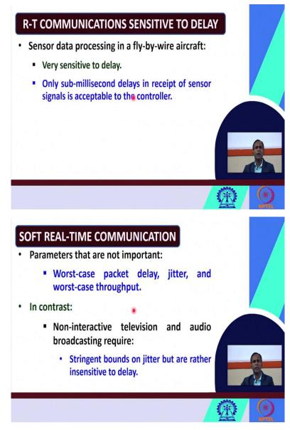
Now, let us say this real time communications sensitive to delay, how? I have they told you that the soft real time communication they do not consider few of the parameters, some of the parameters are not important for them, for as worst case packet delay, jitter and this worst case throughput.
