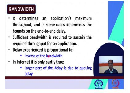
So, one more definition we must see that is bandwidth. You know that bandwidth determines what? It determines the applications maximum throughput and in some cases determines the bounds on the end to end delay. Bandwidth normally determines the applications maximum throughput and in some cases bandwidth also determines the bounds on the end to end delay. So, sufficient bandwidth required to sustain the required throughput for an application.
