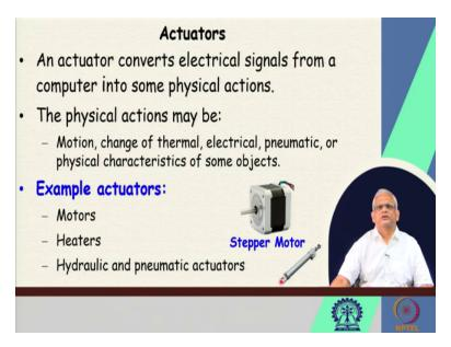
Now, what about the actuators? There are also many types of actuators which are used in these embedded applications. The actuator says we have been saying that they take the electrical signal from the computer and perform some physical action. For example, the physical action can be in terms of motion or change of thermal characteristic, heating, let us say, or cooling, it may be change of electrical characteristic, it may be pneumatic or physical characteristic of the object.
