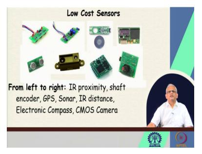
These are some examples of low-cost sensors. From left to right, we have the IR proximity, so proximity sensors, infrared based proximity sensors, soft encoders, GPS, IR distance, electronic compass and CMOS camera. So, these are some of the sensors that might be used in embedded application. But then there are a large number of sensors, just given here a few examples of low-cost sensors.
