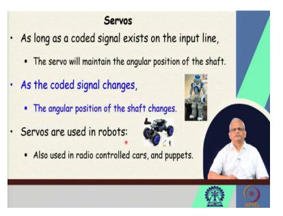
Based on the computation by the computer, it may want to change the direction of the robot, for example, so it will give a command, a coded command to the servo which will change its angular position and based on which the robot will appear to change its direction of movement. And the servos are also used in radio-controlled cars, puppets and so on.
