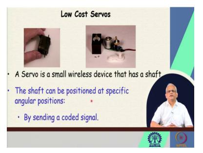
This is another type of actuator are the servos, very popular in embedded applications. A servo is basically a small wireless device that has a shaft. Look at here the shaft here. So, the shaft can be positioned at specific angular position based on some commands. The commands are basically
