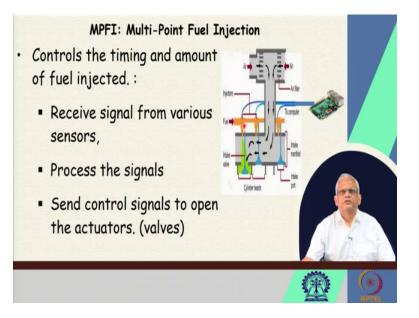
Now, let's look at one typical example of a real time system is this multi-point fuel injection. As I was saying that this MPFI is now a mandatory requirement for all cars. The conventional mechanical fuel injection carburetor system is inefficient. And therefore, to make the cars efficient, reduce pollution level, the MPFI has become mandatory.
