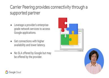
Carrier peering enables them to access Google applications such as G Suite by using a service provider to obtain enterprise-grade Network Services that connect their infrastructure to Google. When connecting to Google to a service provider. They can get connections with higher availability and lower latency using one or more links. As direct peering Google does not offer an SLA with carrier peering but the network service provider might.
