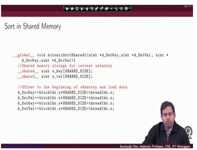
So we are going to do the sorting based on the key values. Now we provide the implementation of bitonic sort on shared memory. So we will have each thread loading 2 values to a shared memory and proceeding through the different stages of the sort. So we define 2 of these shared memory segments one for the storing the key values and one for storing the one for storing the keys and one for storing the values here.
