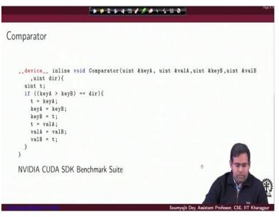
Now these are simple codes that we have taken from NVIDIA CUDA SDK benchmarks right and so first thing we highlight here is the comparators code. So what we have is 2 inputs now we are writing a general situation here. So we have 2 inputs with key value pairs right. We have 2 inputs with key value pairs and we also provide a direction and then for the inputs we compare the key and then we compare it with the direction.
