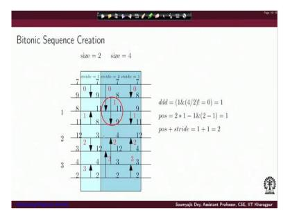
Now this is also an example through which you can identify how everything is going on. So here we have actually noted down in the as a part thread activity that thread Id 0 is performing, this operations thread Id 1 is performing, this comparisons thread Id 2 is performing, this comparisons thread Id 3 is again performing this comparison so on and so forth. And we have also done some example computations of triple d position, position + stride etc.
