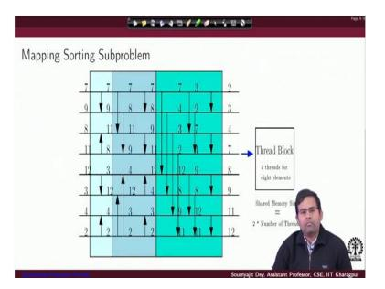
So fundamentally we need to also identify that what is the size of the thread block? As we discussed that since 4 threads are going to do the job in this case. So if I have an 8 element input I would require half the number of threads okay but what is the shared memory size is going to be same as the input size here for each block right. So it is going to be twice of the number of threads right.
