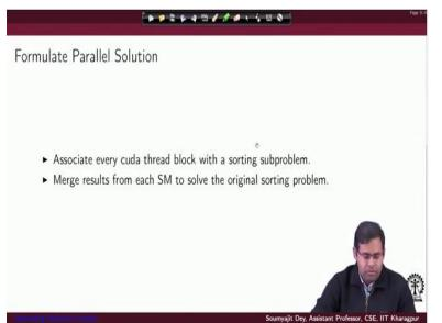
So overall we can summarize like this that associate every cuda thread block with a sorting subproblem. So essentially if we have a significantly large sized array to sort you define cuda thread blocks for each of the sub arrays and then you apply the merge on the results for the different thread blocks that you derive. So at the end you have to actually merge results from each of the SMs and solve the original sorting problem.
