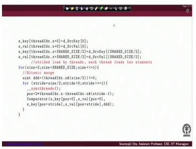
So once we have figured out that this is the location from which we are considering the threads to load the values into the shared memory. So now the pointers have been shifted to the offsets. So now you can just access the location with this as the base shifted by 0 for the source key and the source value right and you write it back to the shared memories location only with the thread Idx offset.
