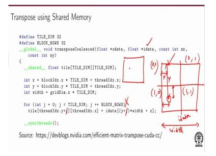
So let us get on with the first example on computing transpose operation on matrix while exploiting shared memory optimization. In the program example that we have provided in our case we have written the tile dimension and the number of block rows to be equal. So to be more specific here let me just give an example what we mean by this 2 parameters. So essentially just like our earlier example where we exploited share memory if you remember it was in matrix multiplication.
