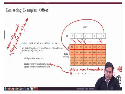
Now consider a small difference here in the program. So let us look into the earlier program once again so earlier program was this atid is atid +1. In this program we are providing an extra parameter here access with offset and the offset value is s. So you compute using normal notion the tid and then what you do is you do the access for atid +s as location right.
