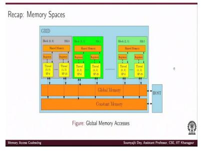
So before getting into the detail of that let us first do a small recap on the hierarchy in the GPU memory. How the different memory segment are organized and how really the global memory is accessed by the computing threads inside an SM. So as we have discussed earlier when a kernel launches essentially a grid of thread blocks are launched. Multiple blocks can reside inside one SM as decided by the high level scheduler of the GPU and it depends on the size of the blocks.
