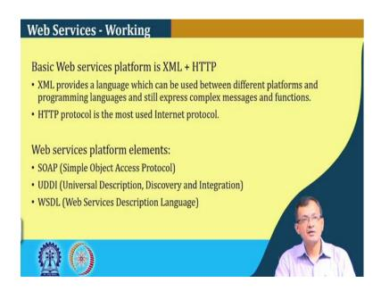
So, if you look at the web service working so, it is XML plus HTTP. XML is the encoding part and the HTTP is the carrier of the things. So, XML provides the language which can be used between different platforms and programming language and still
