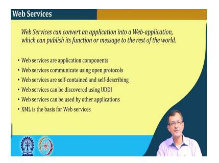
So, that is the big picture sort of thing and also we see that web services can convert an application or what we say a sort of a coat un coat proprietary application is way well enabled application right which can be published its function and messages to the rest of the world. That is the beauty of the web service philosophy. So, it can be published in the
