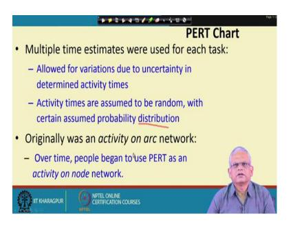
The PERT chart, the tasks have uncertainty and therefore, multiple time estimates were used for each task. This allowed for variation in the activity times that is completion times of the task, the preceding task and so on. This can be accommodated represented in the PERT chart and statistical inferencing can be drawn from the PERT chart. The activity times are assumed to be random with some probability distribution.
