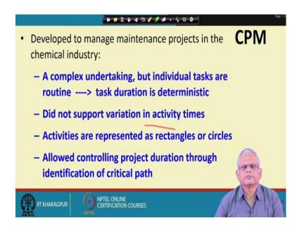
The CPM, the Critical Path Method, as you are mentioning it was developed for managing maintenance project in chemical industry on DuPont. Here the maintenance is a complex activity. There are many tasks here, but the tasks are routine and therefore, the task durations are deterministic. And therefore, CPM did not required to use variation in the activity times and the times there are estimated for activities or constant times.
